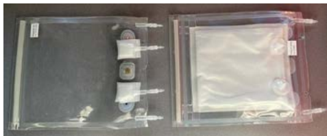
FIGURE 1 The single-use SCINUS adherent culture bag (left) and the suspension culture bag (right), with incorporated sensors to the right
