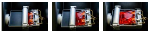
FIGURE 2 Volume expansion of the bag. Minimal volume (left), half the volume (middle) and maximum volume (right).
