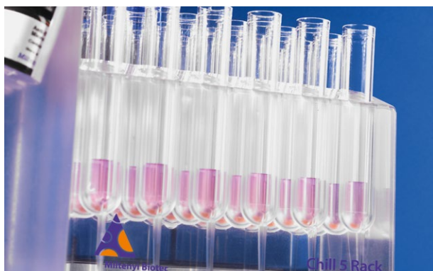
Figure 4: MACS Chill Rack can maintain the temperature of the samples at 4 °C.
